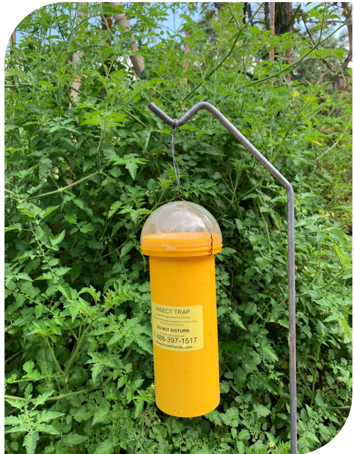
1a - Psyllid trap from 3D printer used to monitor potato psyllids in tomato fields. The trap was designed by James Snyder, FDACS-DPI, based on a concept from early work by Dr. Dyrana Russell, FDACS-DPI. This trap preserves insects for DNA analysis and eliminates most of the by-catch and all the sticky mess associated with standard yellow sticky cards. Photo by Doug Restom-Gaskill, USDA/CAPS
