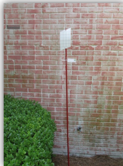
Figure 1: Formosan termite alate trap
