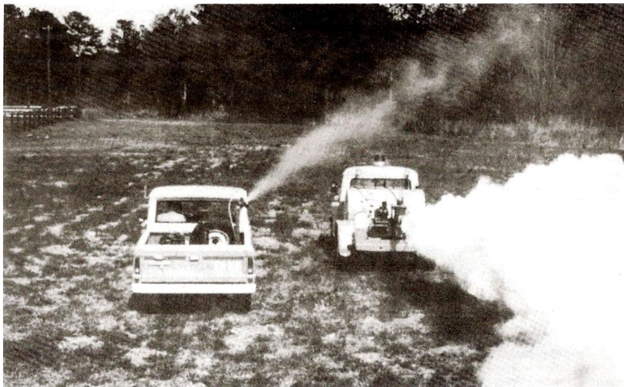
Figure 25. Comparing ULV (left) and Thermal Fogging (right)
